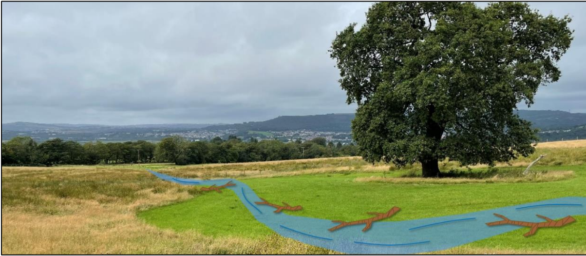
Figure 5 Illustration of the proposed features including breaking out the ancient underground drain and bringing water flow to the surface.
