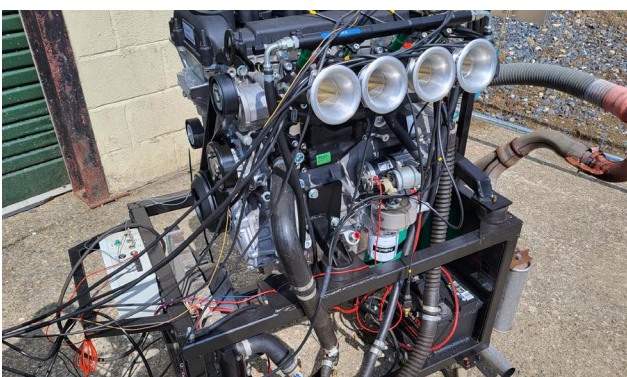
4 cylinder Hydrogen Internal Combustion Engine (HICE) test rig at Systemau Injan PlusZero Cyf.
