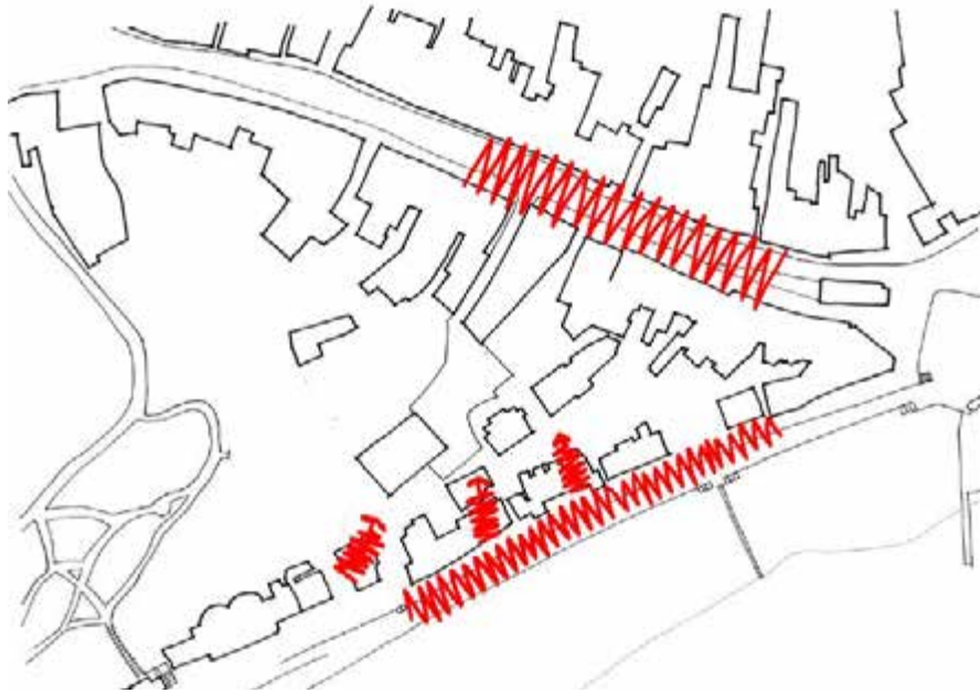
Fig 9: Noise Map Map noise sources to inform building and site layouts © Mat Jones
