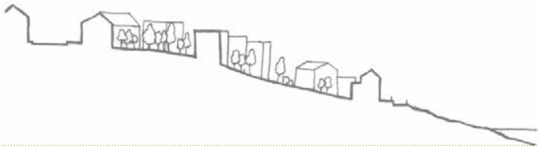
Fig 3 Site section Section drawings cutting through the site demonstrate the impact of any slope and landscape features © Mat Jones
