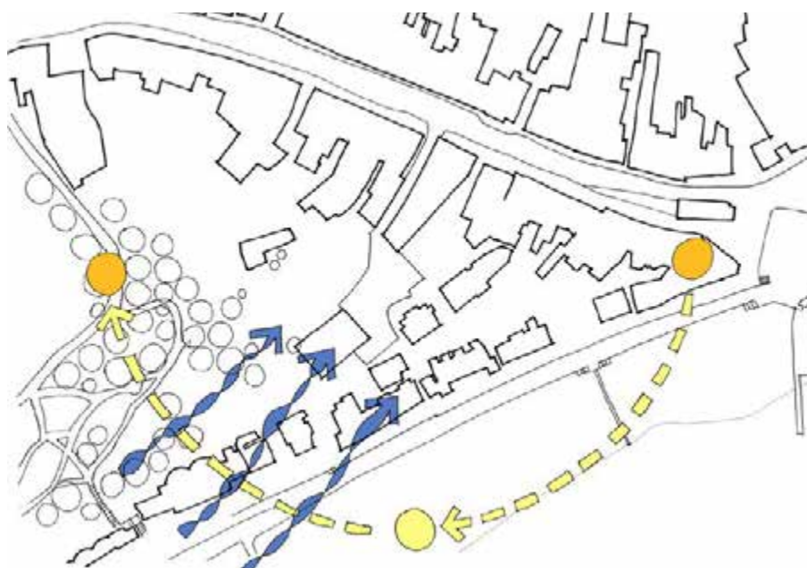
Fig 4 Sun path and wind Identifying the sun path and prevailing wind can help with site planning © Mat Jones
