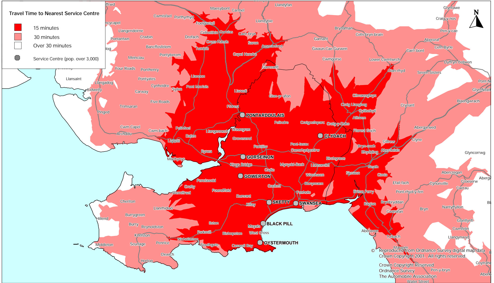
Car access to service centres in Swansea. Produced using isochrone generating software, combining isochrones to individual locations to form an overall access isochrone.
