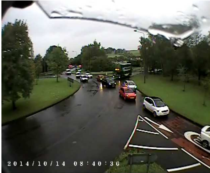
Figure 4.7: CCTV image of blocking back from A468 Exit Bassaleg
