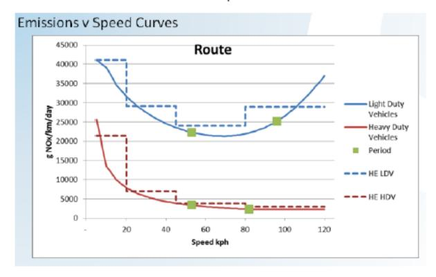
The above graph shows the profile of both light duty vehicles via the blue line (cars, vans) and heavy duty vehicles via the red line (HGVs and buses, coaches).
