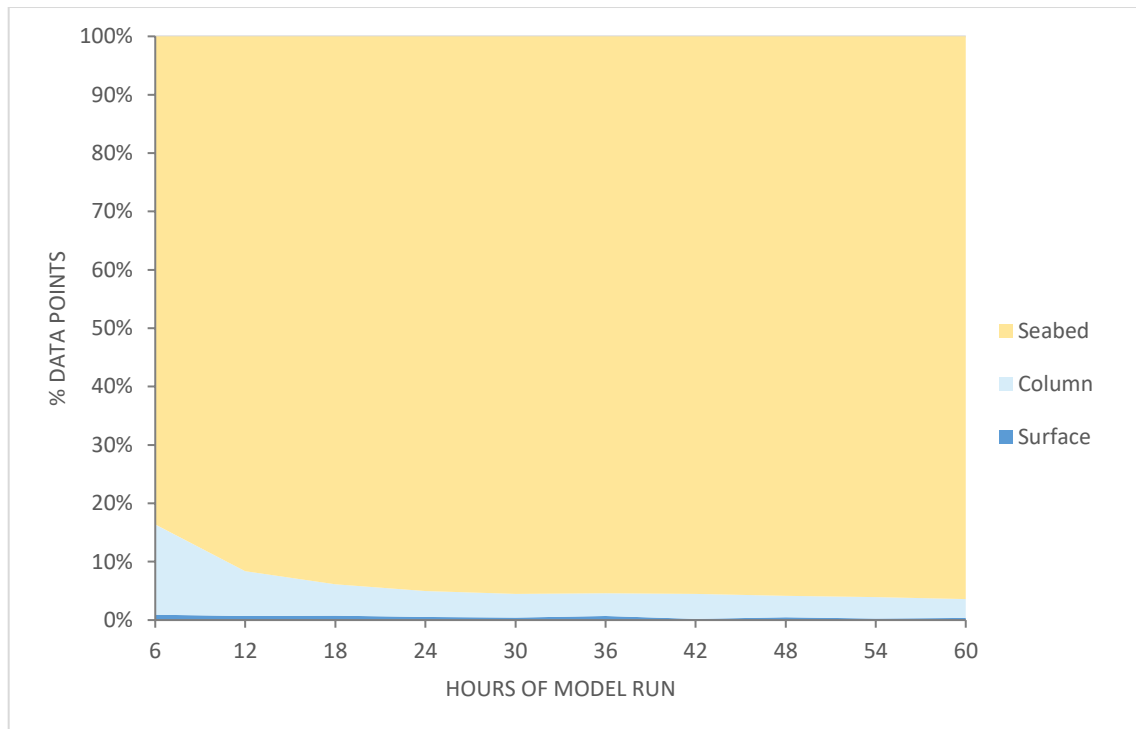
Figure 4.30 Stacked area chart showing the percentage of model data points that were in the water column, seabed and surface, throughout the model run for disposal site LU168 (Milford Haven Two).
