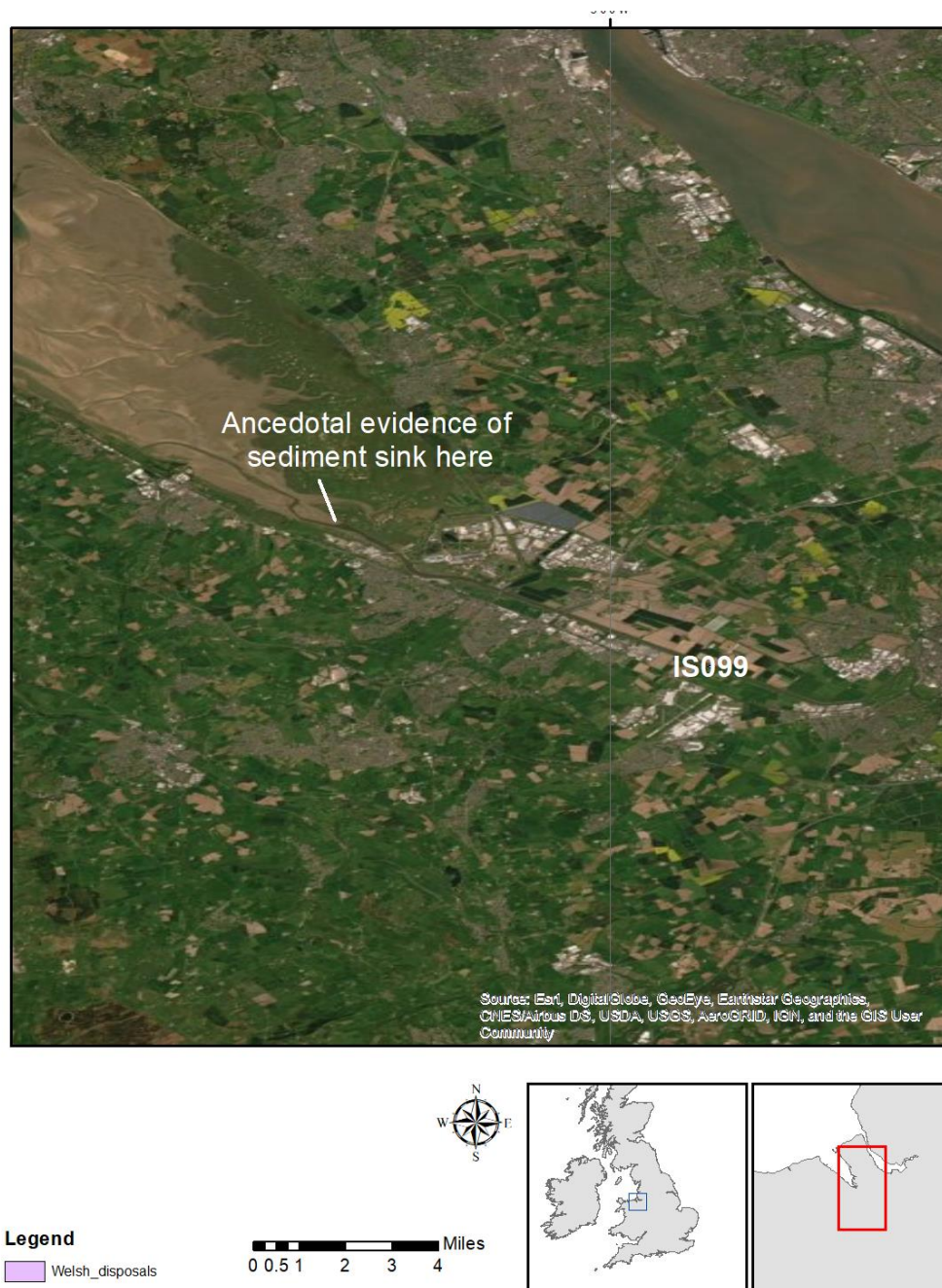
Figure 4.8: Satellite imagery showing the location of Broughton (IS099) and the location of a suggested sink for sediment.
