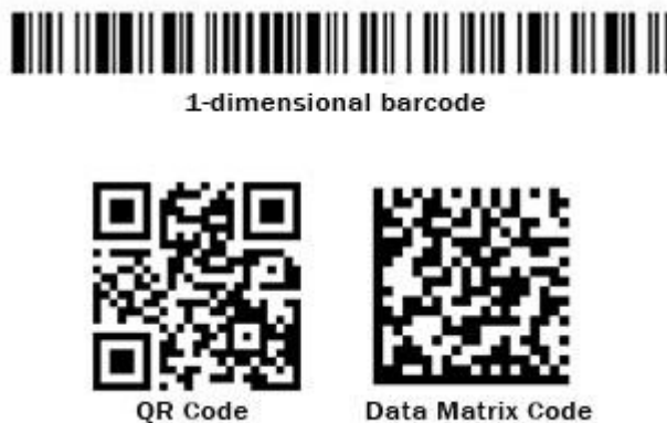
Figure 2. 1D barcodes vs 2D QR code and 2D Data Matrix code. Data Matrix codes can be printed at lower resolutions and smaller sizes, compared to QR codes, making them more favourable for drinks packaging. Source 18 .
