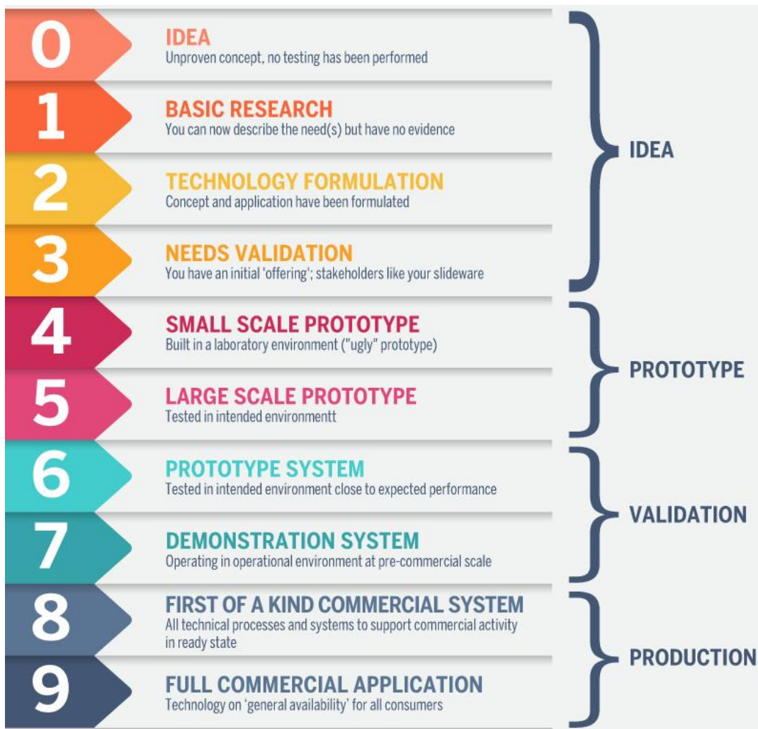
Figure 3. Example scale of technology readiness levels 34
