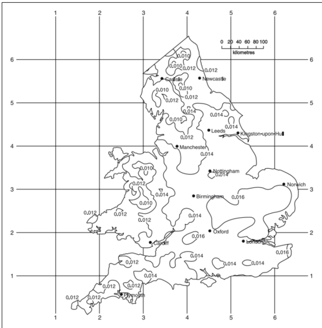
Diagram 2 Rainfall intensities for design of drainage from paved areas and underground rainwater drainage (litres per second per square metre)
