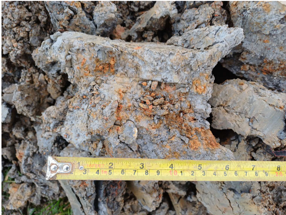
Photograph 8: Evidence of clear prominent ochreous mottling in a greyish matrix within the sub-soils of TP05.
