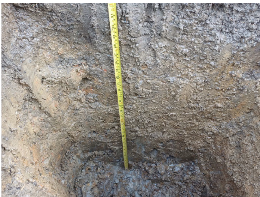
Photograph 7: Evidence of water in the topsoil perched on the underlying slowly permeable sub-soils with abundant diffuse mottling becoming clear and prominent towards the base.
