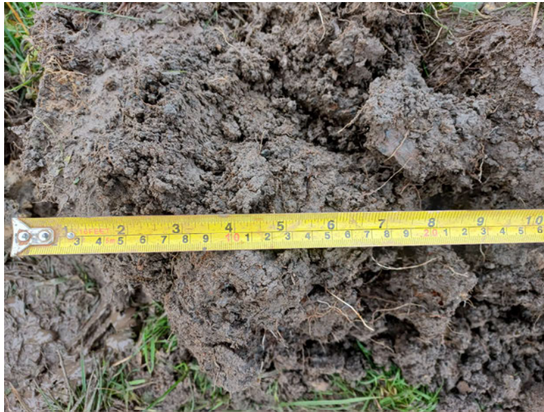
Photograph 5: Clay topsoil from the western site parcel with fine sub-angular blocky to granular peds and frequent grass rootlets creating bio-pores. Faint mottling can also be seen.
