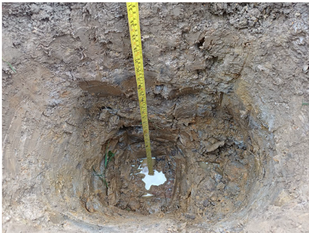
Photograph 9: Groundwater seepage pooling in the base of TP08. Soil profile also shows evidence of mottling within the greyish brown matrix.
